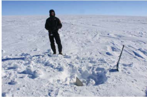
Corner reflector (CR) Calibration of RCS attenuation by snow/ice cover
